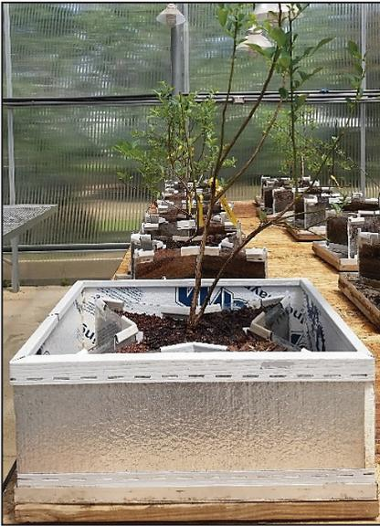
**Figure 2.** To exclude light and protect the root system from temperature extremes, exterior walls were constructed from foam insulation board and placed around each Horhizotron™.
