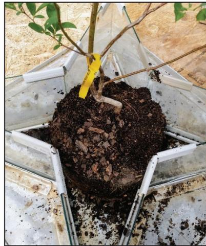
**Figure 1.** Horhizotron™ has four wedge-shaped quadrants that extend out from the root ball. Quadrants are constructed of glass panes connected by vinyl j-channels. The aluminum base onto which the glass panes are attached is fastened to a treated wood frame.
